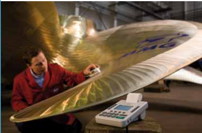
Roughness measurement on ship propellers (Mecklenburger Metallguss)
