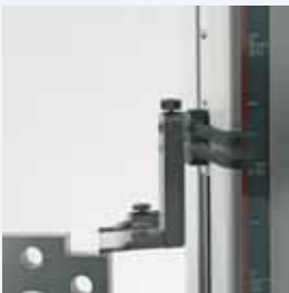
Probe contact with the motorized measuring carriage.
