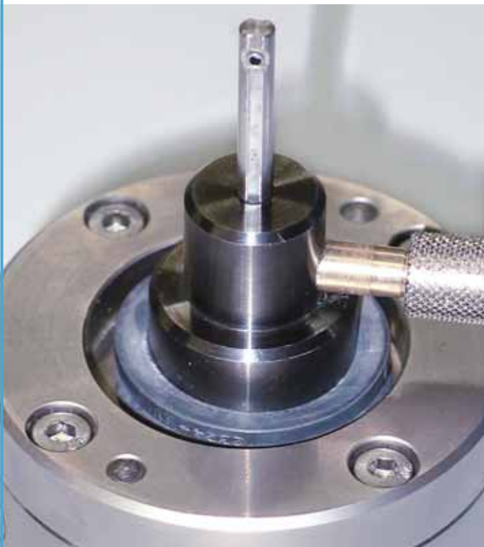
Jet air plug gage with floating bearing
