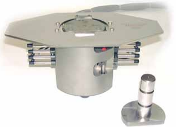
Electronic multi-gage measuring device to test 6x \phi and perpendicularity
